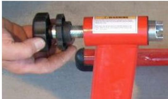
6. Insert the axle end first that does not have the handle on it as shown below.
