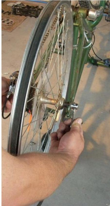
4. Make sure the wheel is equidistant from the frame. This is a very common mistake. Notice in the picture below how the gaps between each side of the wheel and frame are the same size. You need to do the same comparison check.
