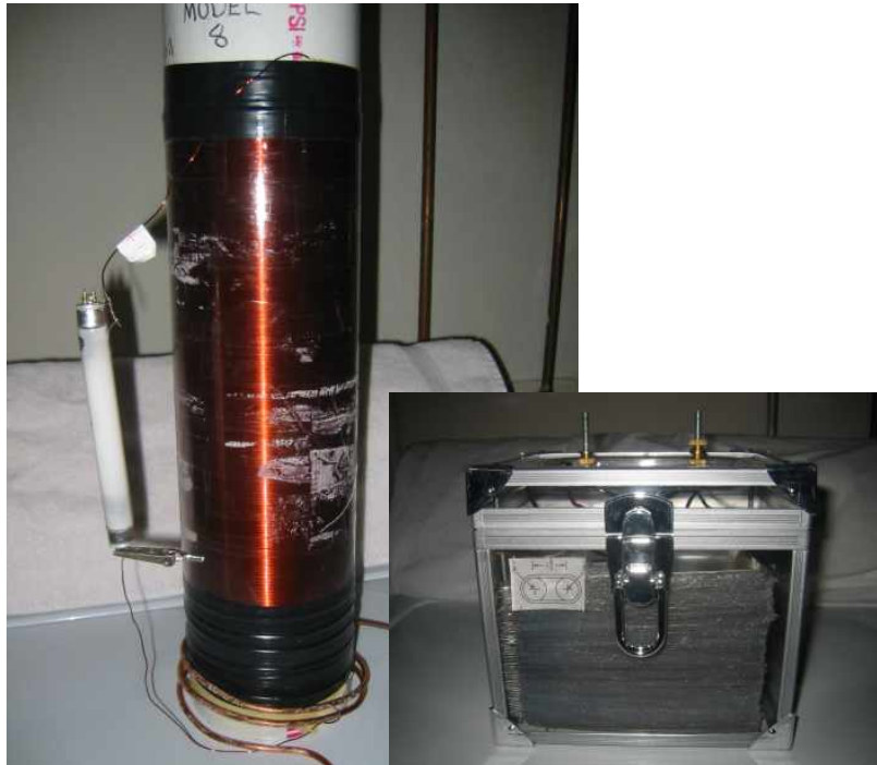
Tesla Coil using a 4" PVC Pipe
