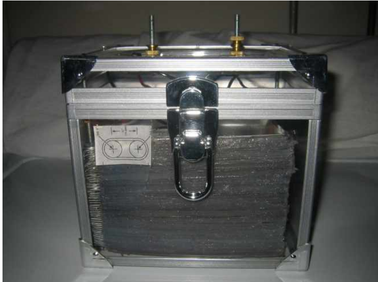
A multi-stack HV Capacitor using clear 4 mil mylar.
