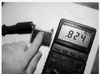
Two cells measures .824 vDC
